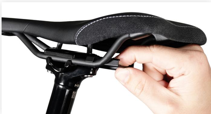
**1.** Position the upper part of the holder between the saddle rails. Do not remove the nuts and hold them firmly if necessary.
