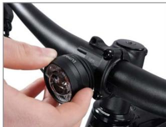
2. Tighten the lower screw of the stem clamp.
