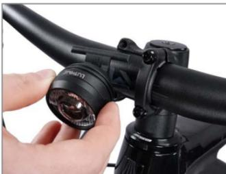
1. One of the stem clamps should be screwed on loosely to the stem. Now insert the lamp into the matching slots of the clamp.
