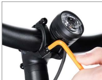
4. Lastly tighten the upper screws of both stem clamps.
