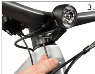
3. Now align the holder together with the lamp and tighten all screws again.
