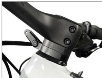
1. Guide the Spacer over the steerer tube. Then mount the handlerbar according to the specifications of the respective manufacturer.
