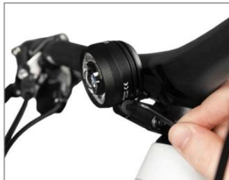
2. Now attach the lamphead to the holder by tightening the two TX15 screws on both sides.
