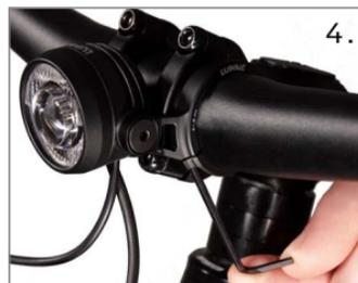
4. Align the lamp correctly and screw it tightly with the allen key 2.5, max. 1Nm
