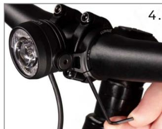
4. Align the lamp correctly and screw it tightly with the hex key 2.5, max. 1Nm
