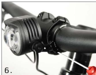
6. Untighten the screw of the mount just a little bit, position the lamp carefully and screw it again with max. 0.5 Nm.
