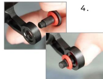
3. Tighten the screw max. 0.5 Nm.
