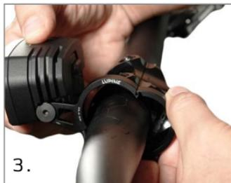
3. Position the lamp together with the clamp at the preferred side of the stem. Then bring both halves of the mount together.
