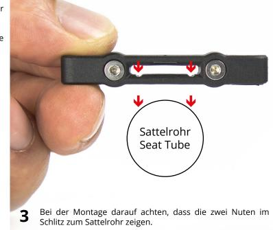
Make sure the two grooves looking towards the seat tube when attaching the seat rail mount.
