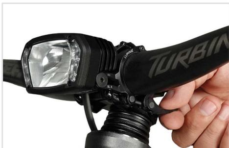
The quick release can be mounted on both sides, depending on the stem width.
