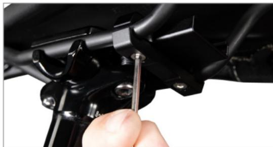
2. Position and mount the lower clamp with the enclosed screws. Important: Make sure that the screws are only screwed in so far that they don't touch the C14 MAG later on.
