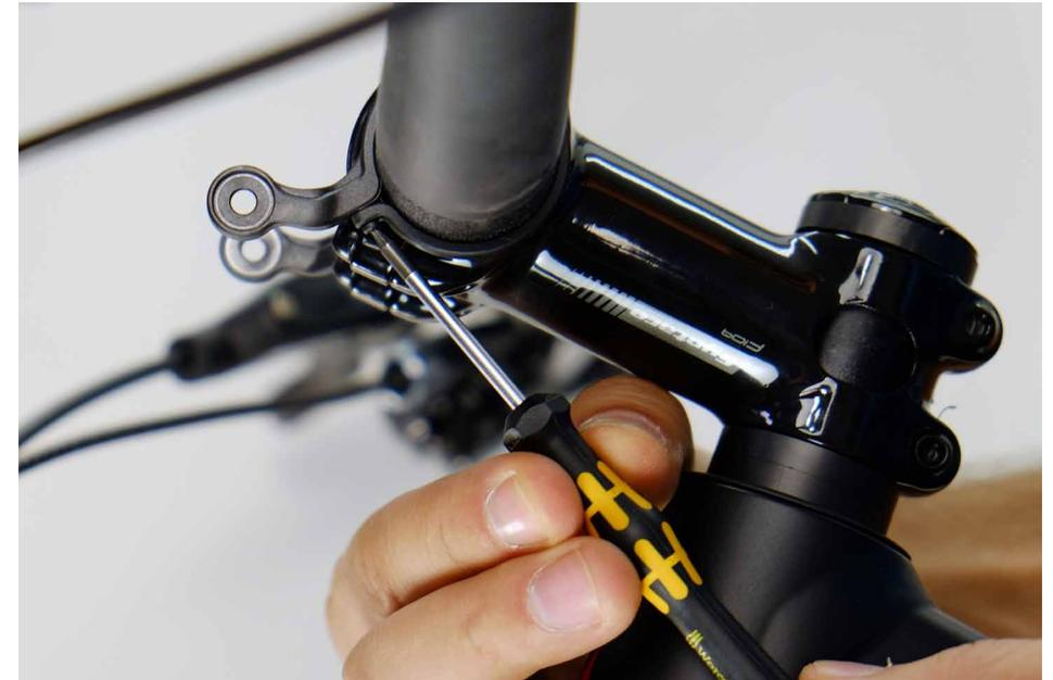
2. Tighten the mount screws firmly in order to attach the mount.
