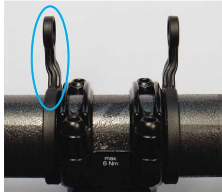
1. The orientation of the mount must be selected according to the stem width.
